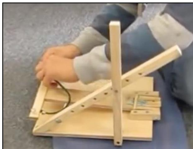
**Description:** (Left) This image shows a different angle adjustment device that uses notches in two wooden sticks.
