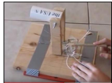
**Description:** (Right) This image shows a launcher with notches cut into two vertical boards that when a rod is placed through serve as an angle-adjusting device. A catapult design is also shown.
