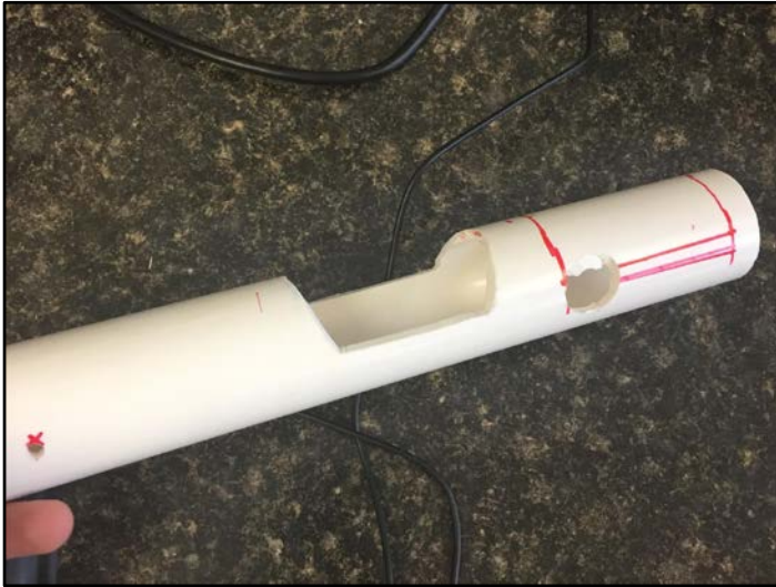
Day 9: 10-23-17 Power sander used to cut holes through side of pipe.
